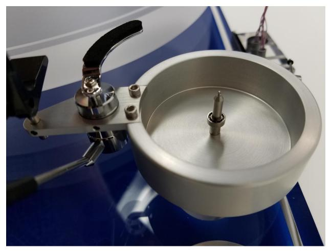
Gently place the pivoting assembly on the pivot and reattach the acrylic cable block to the Velcro on the turntable. Note that if the wires become slightly loose in the acrylic block use the 1/16" hex key to very lightly tighten the screws. Overtightening the screws may damage the wiring.
