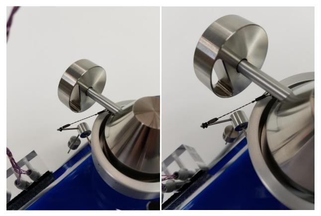
Anti-skate is adjusted by sliding the anti-skate weight up or down the shaft after loosening the lock screw with the .050" hex key. Moving the weight toward the free end of the shaft will increase anti-skate force, toward the pivot will lower anti-skate force.
