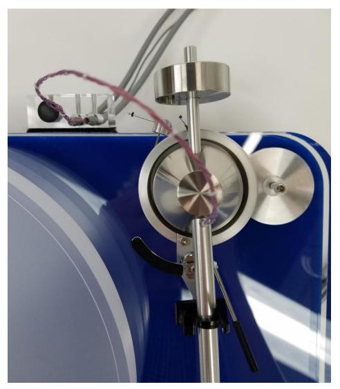
Adjust the counterweight so that there is minimal tracking force. When adjusting the counterweight, pick the pivoting assembly up off of the pivot so that the pivot will not be damaged by the forces and movement naturally caused by adjusting the counterweight.
