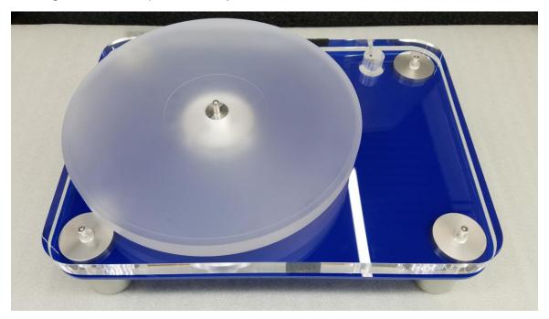
Check that the turntable is level with the bubble level on the platter and adjust the rubber feet at the bottom of the four support pods if needed to level the turntable.
