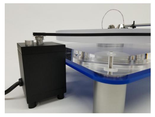
Rotate the platter a few times by hand while guiding the belt on pulley with the other hand until the belt is centered, so it will not fall off or ride up on one of the pulley ridges.
