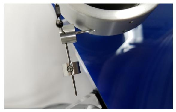
If necessary, adjust the height of the cueing mechanism using the small .035" hex key supplied with the tonearm. When cued down on a record make sure the cue platform goes low enough so it does not contact the underside of the tonearm. When cued up the stylus will be approximately 3/16" from the record surface when the cueing lever is in the up position. You may adjust this to suit your personal taste.
