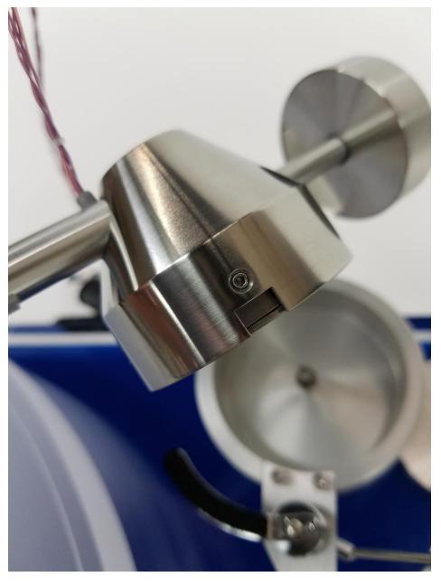
Rotating the azimuth adjustment screw clockwise will raise the right side, counterclockwise will lower the right side when viewed from the front.
