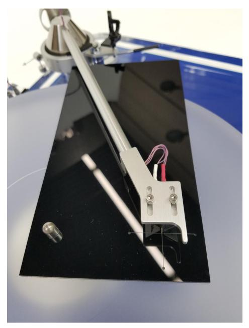
Adjust the tracking force to the cartridge manufacturer's specifications by moving the counterweight. Rotating the counterweight will make it easier to move. Moving the counterweight toward the free end will decrease the tracking force. Moving the counterweight toward the pivot will increase the tracking force. Always lift the pivoting assembly slightly up off the pivot when adjusting the counterweight.
