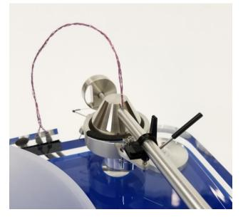
Shape the tonearm wires into a smooth vertical arch and make sure the counterweight is oriented with the cutout on the left side and vertical.
